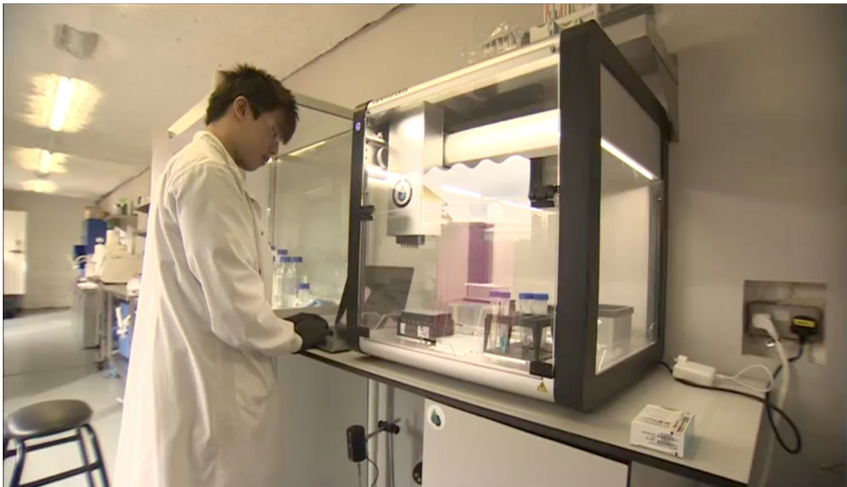
OpenTrons liquid-handling robot OT-2 (similar to many 3D printers) performing DNA test preparation at a OpenCell medical lab in the UK
